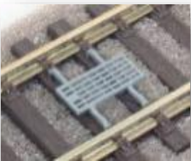
TPWS Train Protection & Warning System
